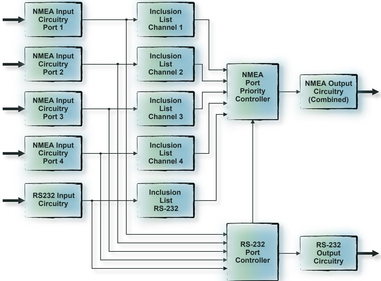
Figure 10 – NMEA Data Combiner signal flow block diagram
